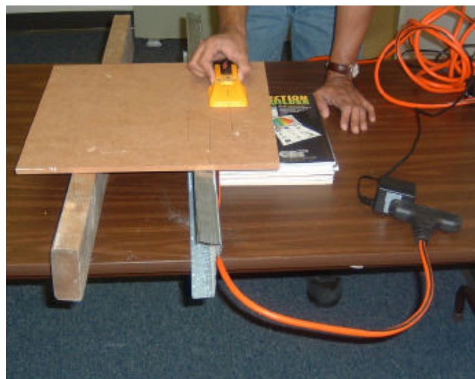
Locating Electrical Wire Behind Particleboard
