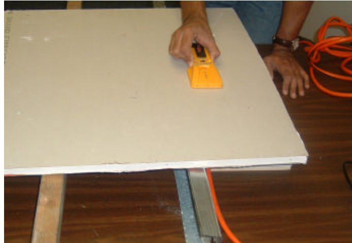
Locating Electrical Wire Behind Drywall
